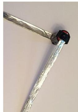
Step 3: Wrap the other end of one piece of foil securely around the base of the lightbulb. Be sure it does not touch the bottom of the bulb.
