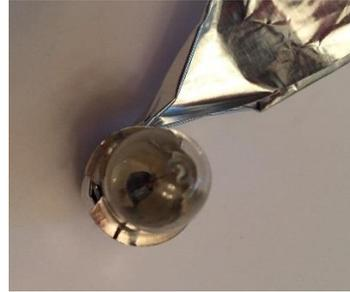
Step 4: To complete the circuit, touch the base of the bulb to the other end of the foil. Tightly hold the foil around the bulb and press down on the foil on the top of the battery to make the light brighter.
